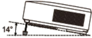
1. Hold the projector, and push the elevator buttons to loosen the feet.
