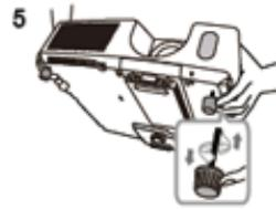
Twist the foot, to finely adjust.
